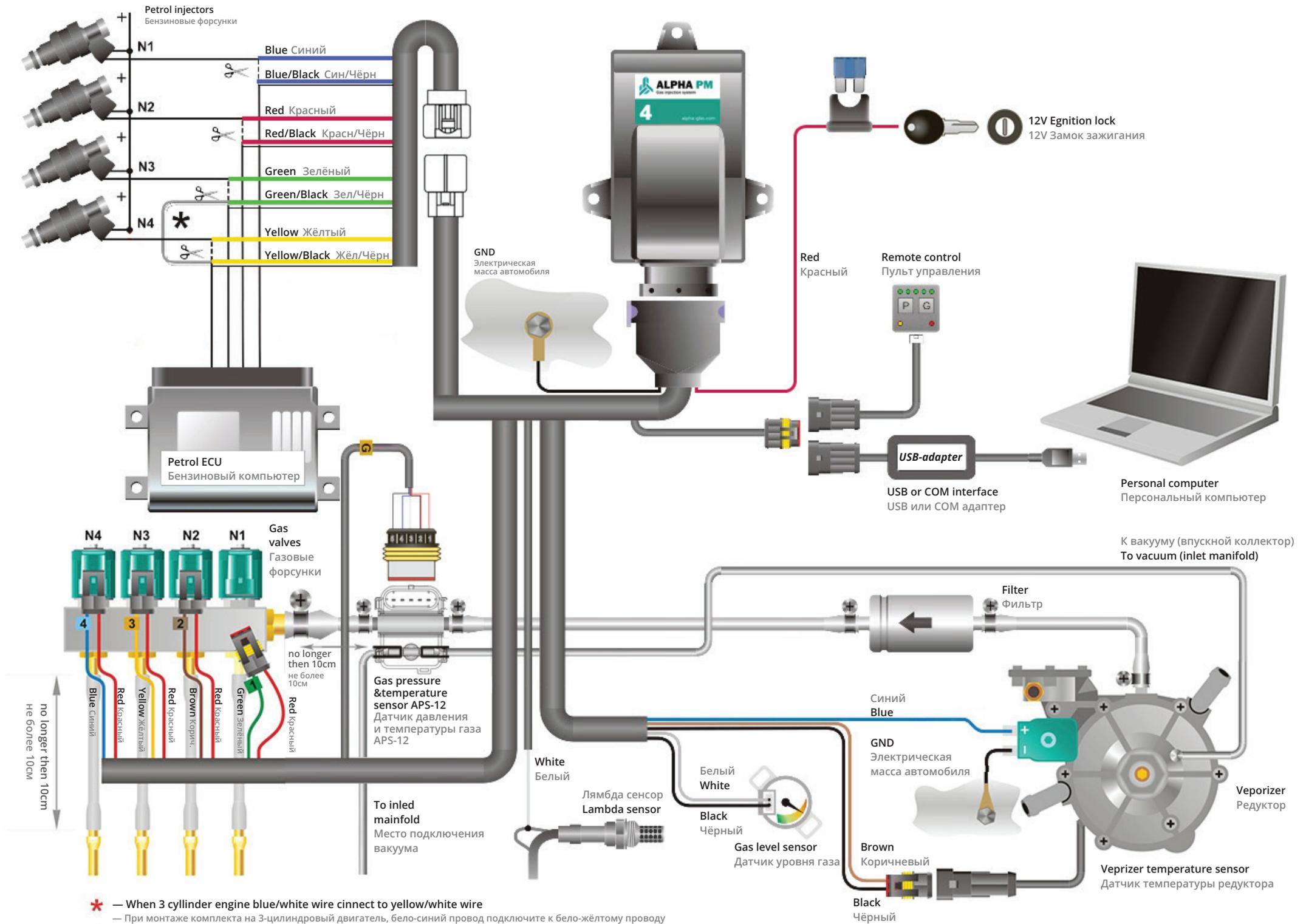
\* — When 3 cylinder engine blue/white wire connect to yellow/white wire
